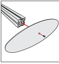
**Base Plate & Extrusion Connection**
