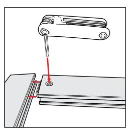
**Extrusion & Lock Connection**
